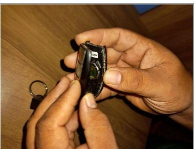
Carefully snap the back cover onto the rest of the remote.
