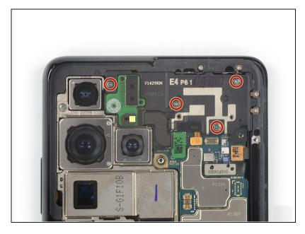
Use a Phillips screwdriver to remove the four 3.9 mm-long screws securing the earpiece speaker and laser AF module assembly.
