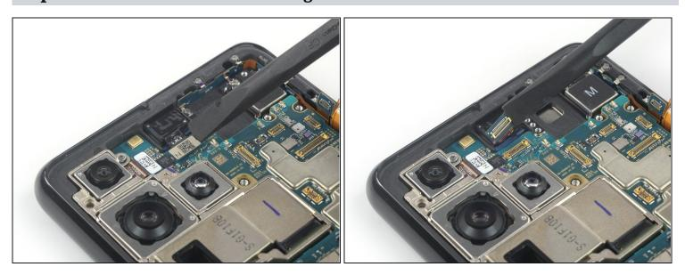
• Use a spudger to disconnect the front facing camera cable by prying the connector straight up from its socket.
