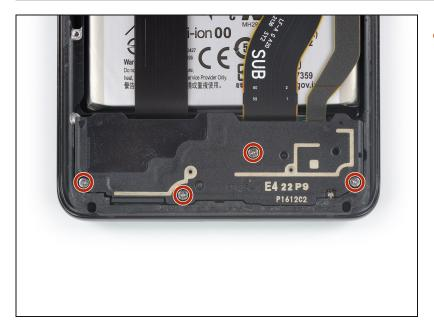
Use a Phillips screwdriver to remove the four 3.9 mm-long screws securing the loudspeaker assembly.
