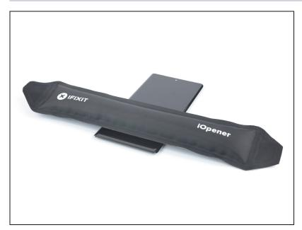
Apply a <u>heated iOpener</u> to the screen where the fingerprint reader is located to loosen the adhesive underneath. Apply the iOpener for at least 3 minutes.
