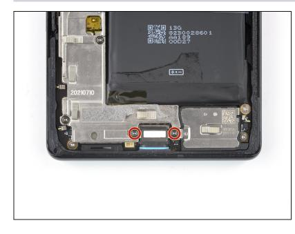
Use a Torx T3 screwdriver to remove the two 5.1 mm-long 3IP Torx Plus screws securing the charging port metal bracket.
