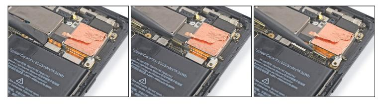
• Use a spudger to disconnect the cables of the wide and ultrawide cameras by prying their connectors straight up from their sockets.
