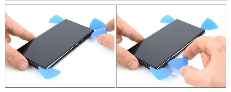
• Insert a fifth opening pick and slide it along the right edge of the phone to slice the remaining adhesive.
