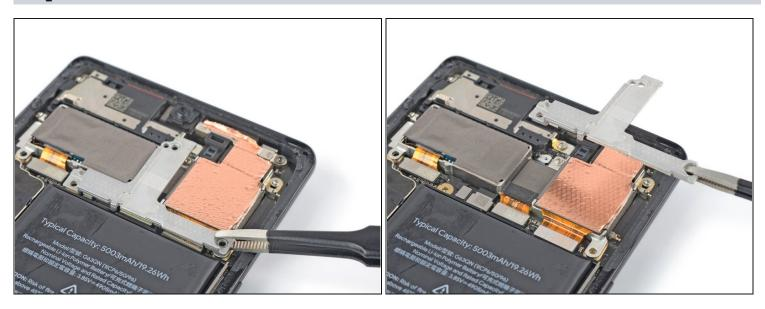
• Use a pair of tweezers to remove the camera connector cover.
