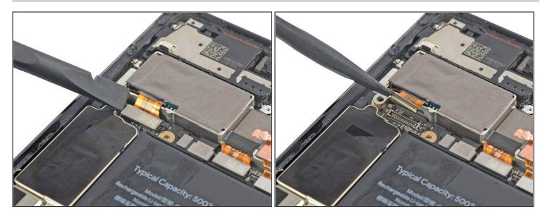
• Use a spudger to disconnect the telephoto cable by prying the connector straight up from its socket.
