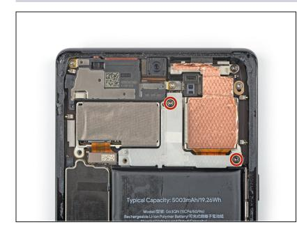
Use a Torx T3 screwdriver to remove the two 5.1 mm-long 3IP Torx Plus screws securing the camera connector cover.
