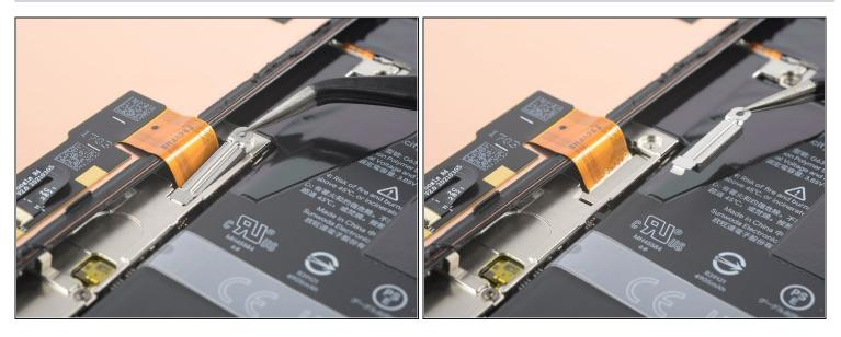
• Use a pair of tweezers to remove the metal bracket sitting on top of the display cable connector.
