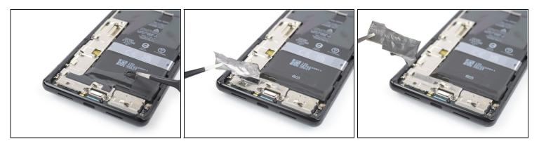
Take care not to puncture or bend the battery with your tool—a punctured or bent battery may leak dangerous chemicals or cause a thermal event.
