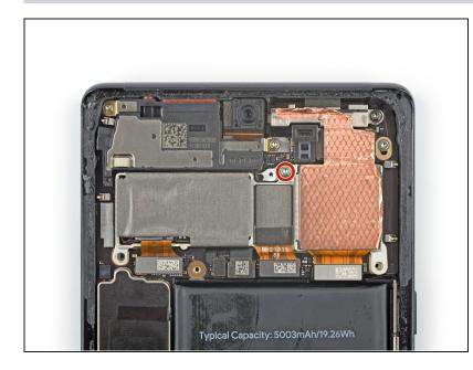
• Use a Torx T3 screwdriver to remove the single 3.3 mm-long 3IP Torx Plus screw securing the camera assembly.
