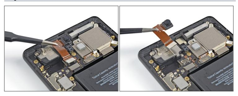
Use your fingers or a pair of tweezers to carefully lift the front camera out of its recess and remove it.
