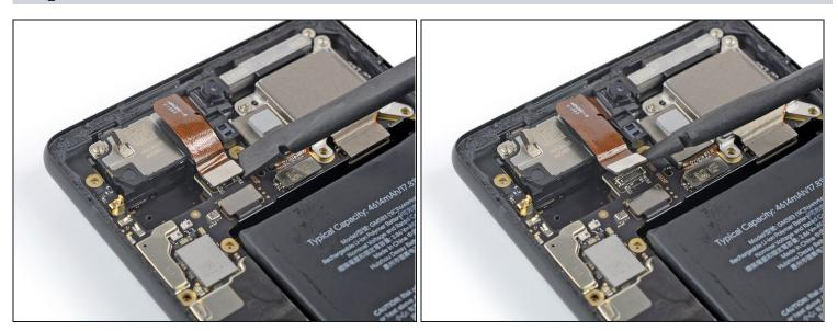
• Use a spudger to disconnect the front camera cable by prying the connector straight up from its sockets.
