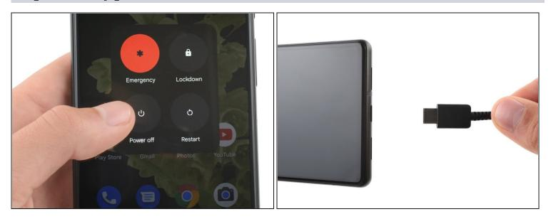
⚠ Allow your battery to drain below 25% before starting this repair. A charged battery may catch fire if damaged.
