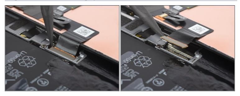
Use a spudger to disconnect the display flex cable by prying the connector straight up from its socket.
