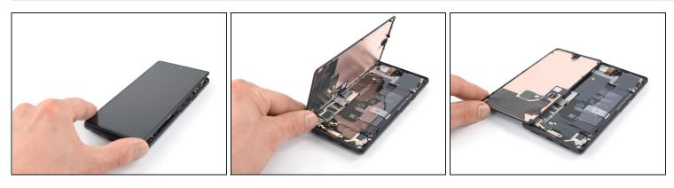
⚠ Avoid straining the display cable during the following procedure.
