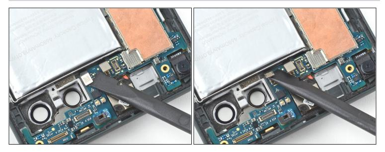
• Use the flat end of a spudger to pry up on the camera flash connector to disconnect it.
