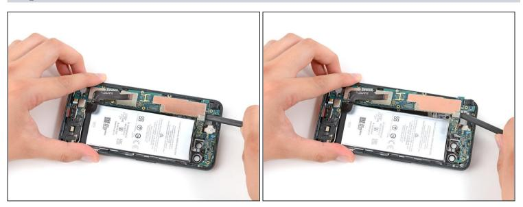
• Insert the flat end of a spudger under the top left corner of the motherboard to lift it from the frame.
