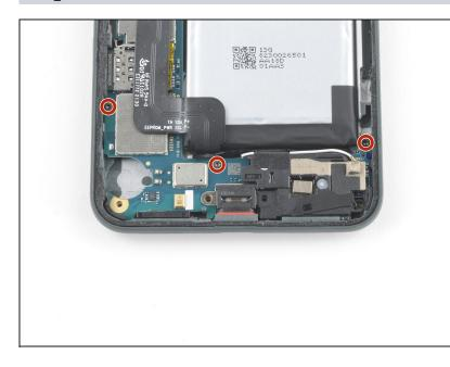
• Use a T3 Torx driver to remove the three 2.9 mm screws securing the motherboard to the frame.
