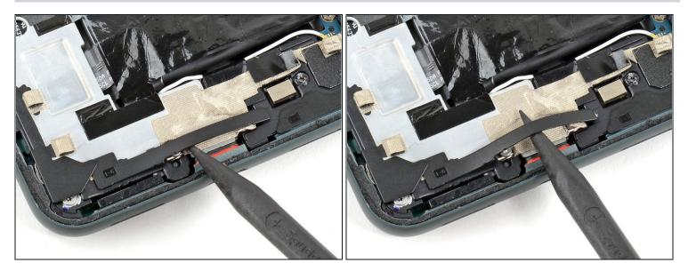
• Use the pointed end of a spudger to pry up on the black plastic cover at the bottom left of the phone.
