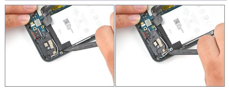
• Insert the pointed end of a spudger under the the screw slot to the top right of the speaker assembly to dislodge it from the frame.
