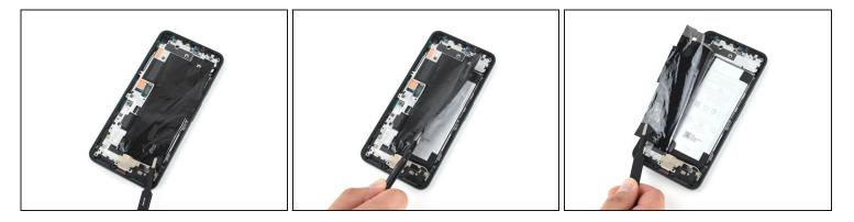
• Use a **blunt** pair of tweezers, or your fingers, to carefully peel back the graphite sheet covering the battery.
