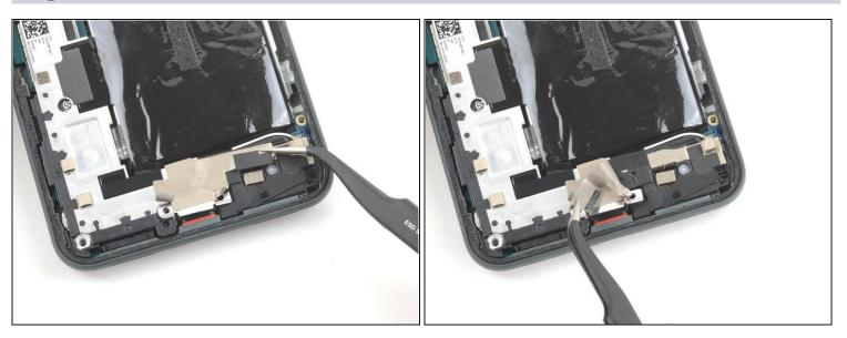
• Use a spudger or a pair of tweezers to peel back the tape securing the charging port bracket to the speaker assembly.
