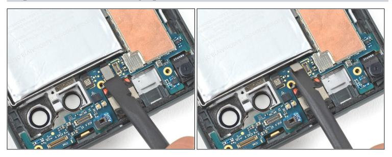
• Use the flat end of a spudger to pry up on the fingerprint sensor connector to disconnect it.
