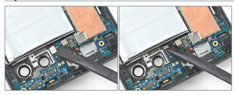
• Use the flat end of a spudger to pry up on the camera flash connector to disconnect it.
