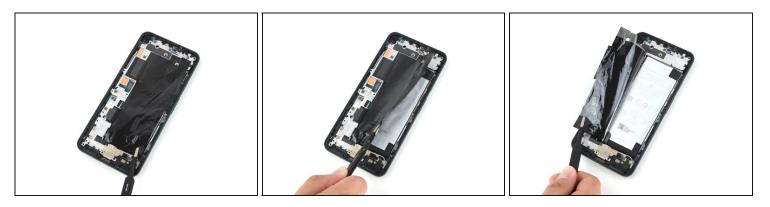
• Use a **blunt** pair of tweezers, or your fingers, to carefully peel back the graphite sheet covering the battery.
