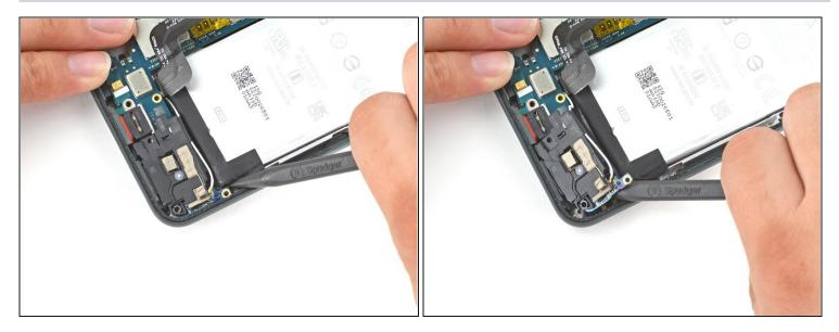
• Insert the pointed end of a spudger under the the screw slot to the top right of the speaker assembly to dislodge it from the frame.
