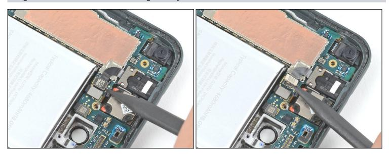
Use the pointed end of a spudger to pry up on the headphone jack connector to disconnect it.
