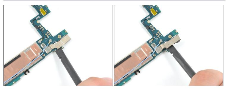
• Use the the flat end of a spudger to disconnect the front-facing camera.
