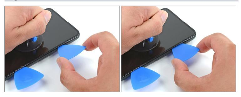
• Insert the tip of an opening pick into the *bezel seam* about 3-4 cm from the top of the phone.
