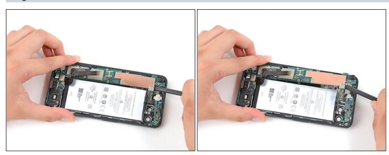
• Insert the flat end of a spudger under the top left corner of the motherboard to lift it from the frame.
