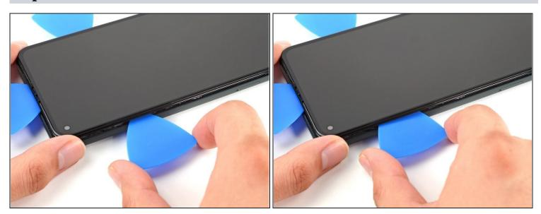
• Insert the tip of an opening pick into the *bezel seam* about 3-4 cm below the front-facing camera.
