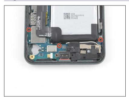
Use a T3 Torx driver to remove the three 2.9 mm screws securing the motherboard to the frame.
