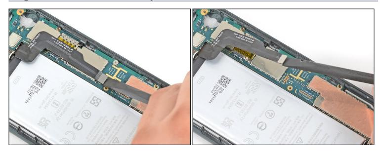
• Use the flat end of a spudger to pry up on the battery connector to disconnect it.
