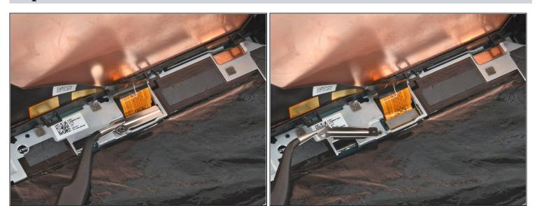
• Use a pair of tweezers to remove the screen connector bracket.
