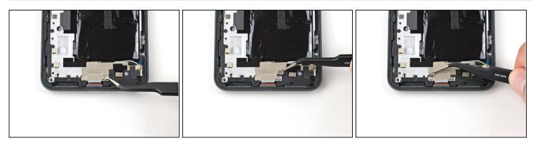
• Use a pair of tweezers to slightly peel back the tape concealing the two screws securing the charging port bracket.
