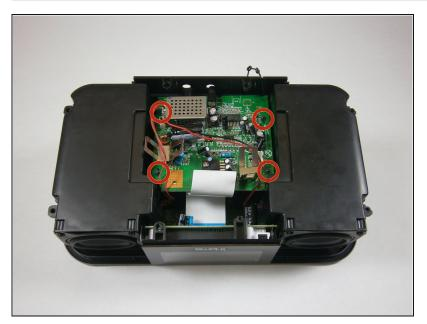
Take out four 14 mm screws using a Phillips #1 screwdriver.
