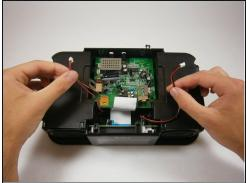
• Use a plastic opening tool to lift the two speaker zip connectors from the logic board.
