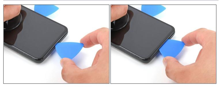
Insert the tip of an opening pick into the *bezel seam* at the bottom of the phone.
