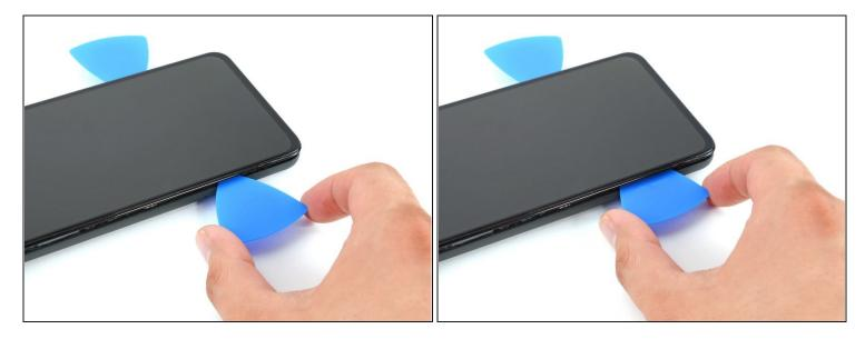
• Insert the tip of an opening pick into the *bezel seam* on the left side of the phone, about 2 cm from the bottom of the phone.
