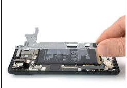
• Carefully lift up the motherboard cover and remove it.
