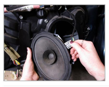
Remove the wires connecting the speaker by pressing the clip and pulling it outward.
