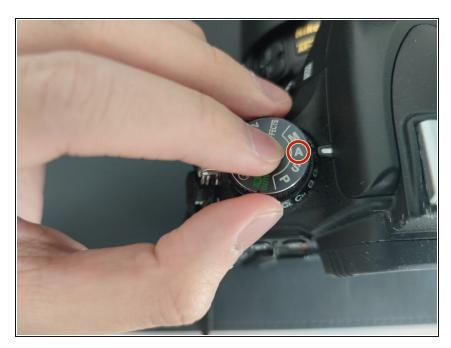
Turn the dial on the left side of the camera to the letter A. This sets the camera mode to "shutter priority."
