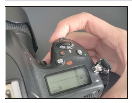
Power on the camera by moving the switch to the "On" position.
