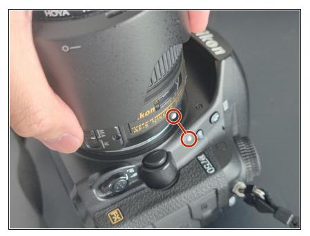
Locate the white dot on the lens and on the right side of the camera.
