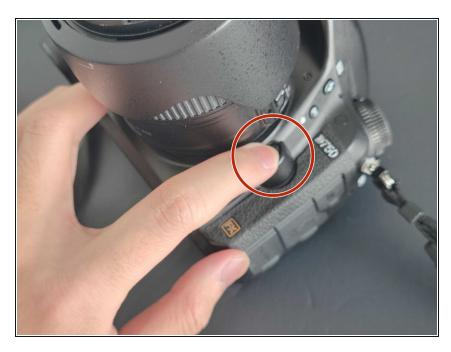
Press and hold the button on the right side of the lens, and while doing so, gently twist the lens to the right in order to remove the lens.
