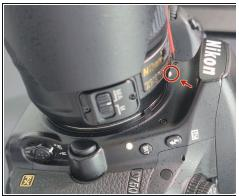
When the cleaning is finished, reinstall the lens. Angle the lens so that the white dots align.
