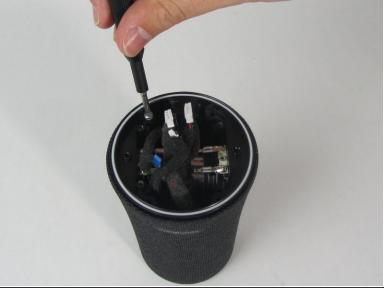
Remove the other four 11 mm screws holding the outer shell in place with a Phillips #1 screwdriver.
