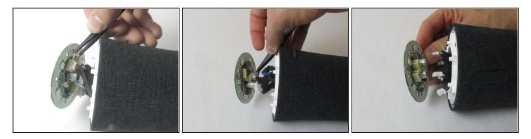
• Use precision <u>tweezers</u> to firmly grasp the five power connectors and detach them from the back of the motherboard.
