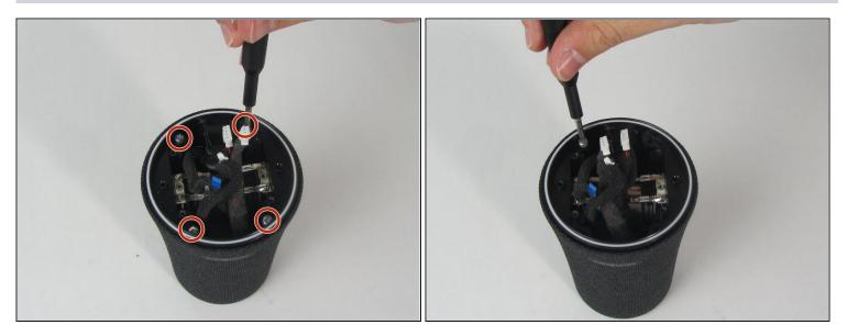
• Remove the other four 11 mm screws holding the outer shell in place with a Phillips #1 screwdriver.
