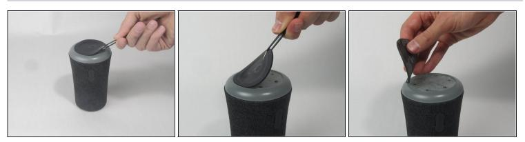
(i) The rubber cover of the speaker is glued down.
