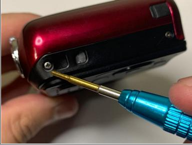
Remove the two 5 mm Phillips #000 screws from the right side of the camera.
