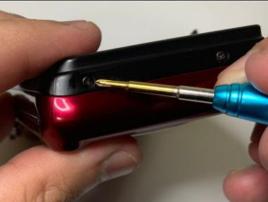
Remove the two 5 mm Phillips #000 screws from the left side.
