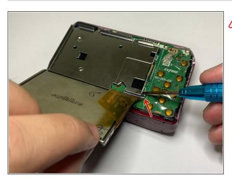
⚠ Lightly push back the white switch holding in the screen cable
