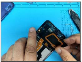
Remove the silver Phillips screws to be able to disassemble the motherboard shields.
