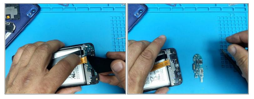
Disconnect the Main flex cable and the coaxial antenna cables and remove the charging board.
