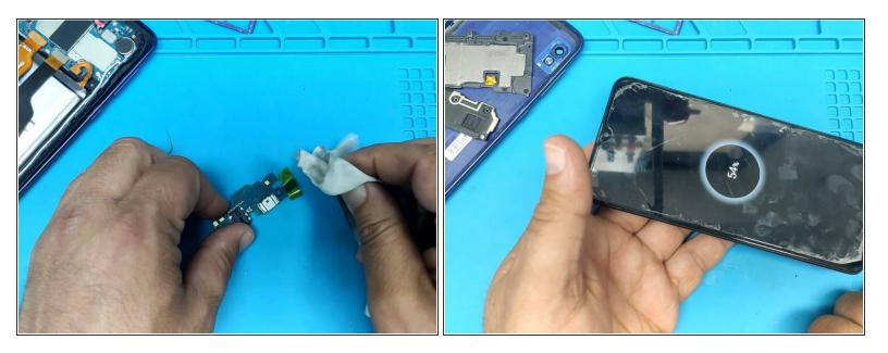
Clean the board and test the device.
