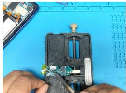
Clean the tin and install the new charging connector.
