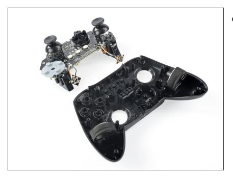
• Remove the mainboard from the housing.
