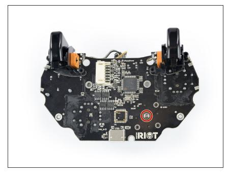
Use a Phillips screwdriver to remove the 7.25 mm-long screw on the mainboard securing the direction pad.
