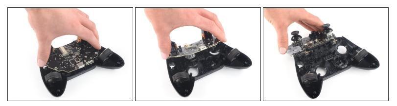
• Flip over the mainboard and place it above the controller housing.
