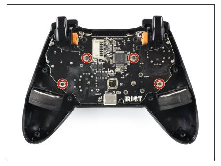
Use a Phillips screwdriver to remove the four 7.0 mm-long screws securing the mainboard.
