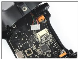
Use a spudger to disconnect the phone connector cable from the mainboard.
