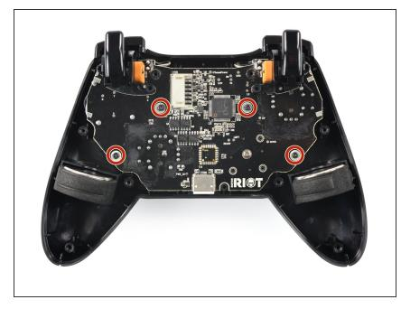
Use a Phillips screwdriver to remove the four 7.0 mm-long screws securing the mainboard.
