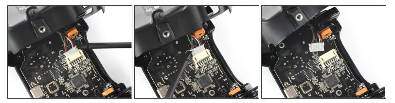
• Use a spudger to disconnect the phone connector cable from the mainboard.
