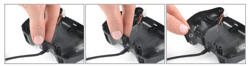
• Pull the screw thread bracket straight up to slide it off of the rails securing it to the back cover.
