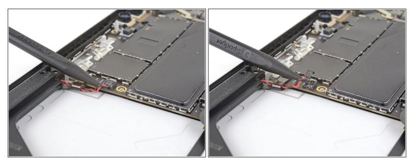
• Use the point of a spudger to lift the left speaker connector out of its socket on the motherboard.
