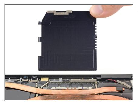
• Remove the heat sink shield.
