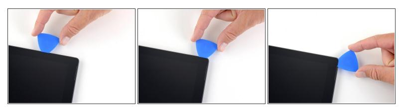
Once you cut the adhesive over the antennas (8.5 inches, or 22 cm, away from the left edge), slide the pick the rest of the way along the top edge of the surface and round the top right corner to slice through any remaining adhesive.
