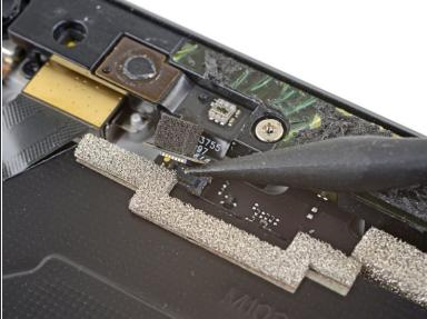
Use the point of a spudger to pry the microphone connector straight up and out of its socket on the motherboard.
