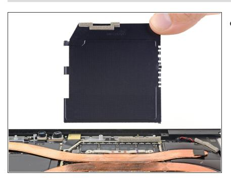
Remove the heat sink shield.
