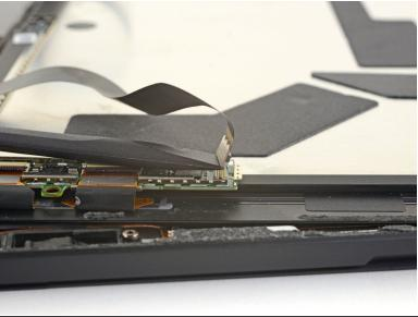
Use the flat end of a spudger to pry the display interconnect cable straight up and out of its socket on the board.
