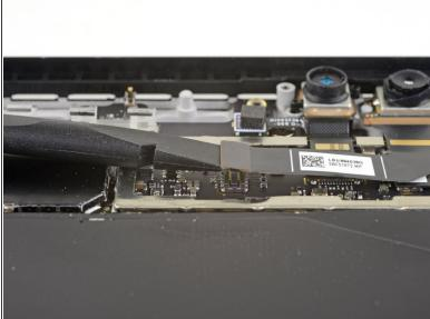
Use the flat end of a spudger to pry the front-facing camera connector up and out of its socket on the motherboard.
