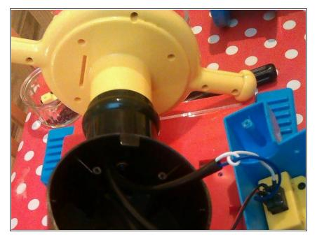
A single screw inside the chimney holds this in place, again you may need a short screwdriver to access this
