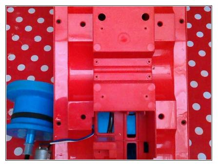
• Over the wheel arches are 2 more plastic panels, they are held in place by screws. Note that the outer screws are a smaller size.
