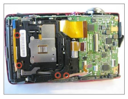
Unscrew the four, 3.5mm Phillips screws that hold down the metal plate.
