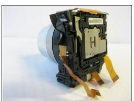
Carefully lift the lens off of the front cover.
