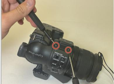
• Remove two screws from each side of the camera (four in total) using a JIS #00 screwdriver.
