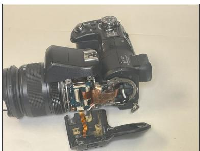
Tighten the two screws using a JIS #00 screwdriver.
