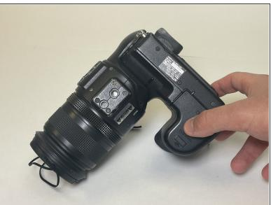
Slide the button back to open the battery cover.
