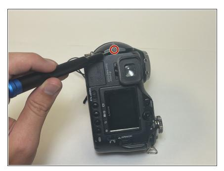
Remove the screw on the back of the turret with a JIS #00 screwdriver.
