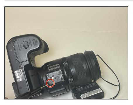
Remove the screw on the bottom of the turret using a JIS #00 screwdriver.
