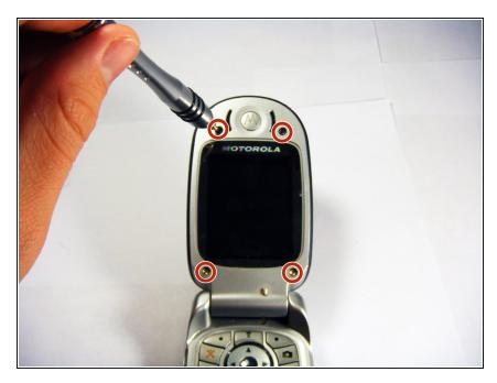
Unscrew the four cover screws using a T6 Torx screwdriver, turning counterclockwise.
