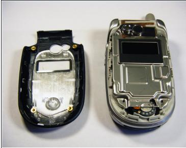
• Loosen and remove the protective cover using a plastic opening tool.
