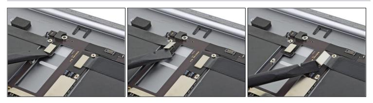
• Use a spudger to pry up and disconnect the two press connectors near the top of the logic board.
