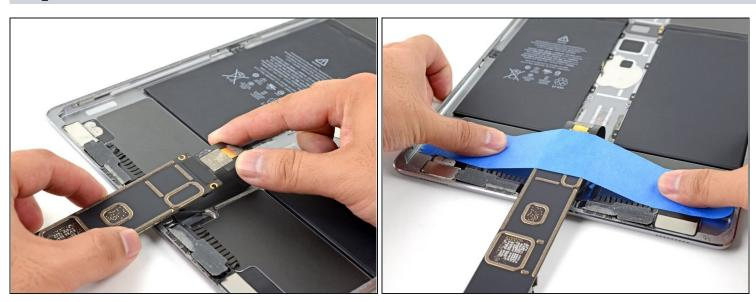
• Once you swing the logic board completely over its flex cable, use a piece of tape to secure the logic board out of the way of the battery.
