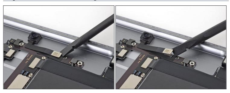
• Use the flat end of a spudger to pry up and disconnect the front facing camera connector.
