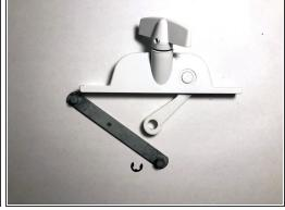
Once the operator is removed, you can use a <u>Metal Spudger</u> or a <u>Flathead 4 mm Screwdriver</u> to force the e-clip out of the operator arm.
