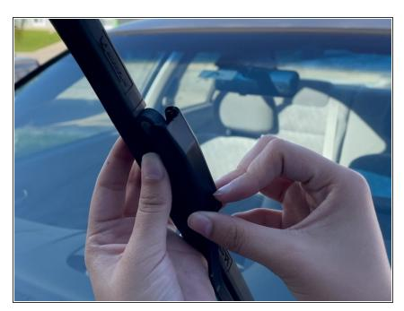
Once the wiper blade is accommodated, close the tab. Pull it upwards to lock it.
