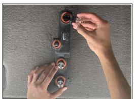
Remove the defective bulb by pulling it up.
