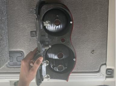
Remove the bulb holder piece from the tail light by gently pulling it up.
