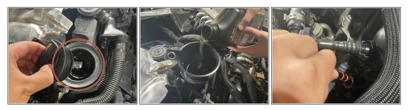
• Unscrew the oil filler cap and add oil to manufacturer's specification. Oil capacity can usually be found in vehicle user manuals. If necessary, use a funnel to limit splash.
