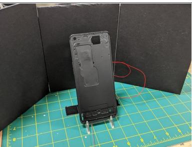
So we replace the PCB with a controlled heater. Remount the vapor chamber, and paint everything black so we can see the pretty thermal images!
