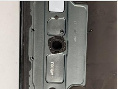
Here we see the cut-out for the acoustic (maybe?) fingerprint sensor. From the chip mounted in the PCB at the bottom of the phone, there is a clear line of sight straight to the underside of the OLED.
