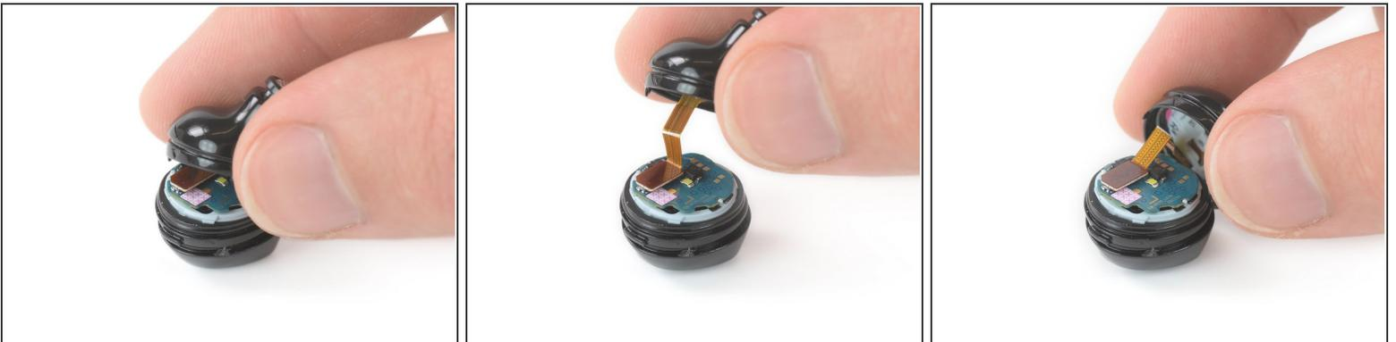
**⚠ Make sure that the flex cable is not under tension during the following step.**
