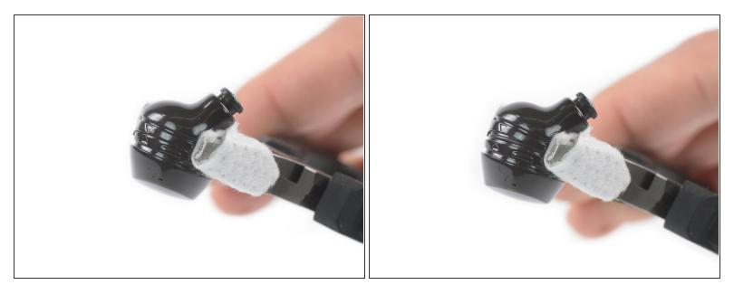
Use a pair of pliers to hold the earbud horizontally along the seam between the upper and lower halves of the case.
