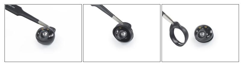
• Use your fingers or a pair blunt nose tweezers to remove the earbud's rubber wingtip by pulling it upwards while slipping it off the earbud.
