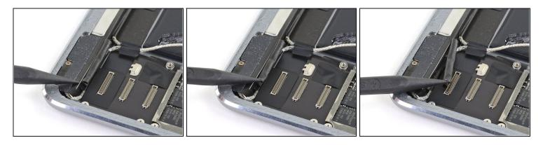
• Use the pointed end of a spudger to detach the foam spacer adhered to the second right antenna sticker.
