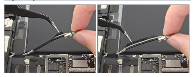
• Use a pair of tweezers to peel up the sticker bundling the left and right antenna cables together.
