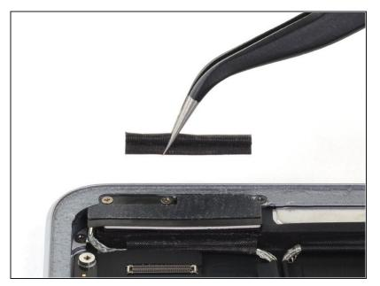
Remove the foam spacer from the second right antenna sticker.
