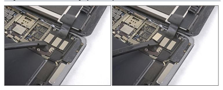
• Use the flat end of the spudger to disconnect the display assembly connector from the motherboard socket.
