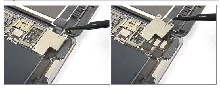
• Remove the display cable bracket.
