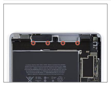
Use a Phillips screwdriver to remove the four 1.9 mm-long screws securing the upper speaker to the frame.
