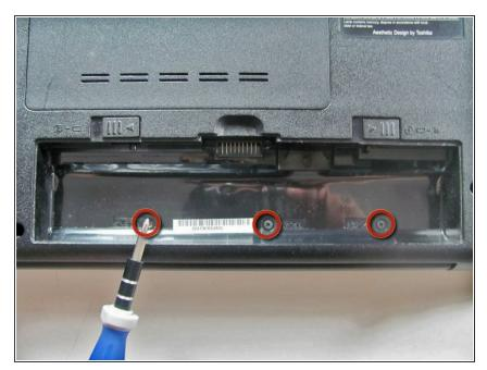
Remove the three 4mm screws with a Phillips #00 screwdriver.
