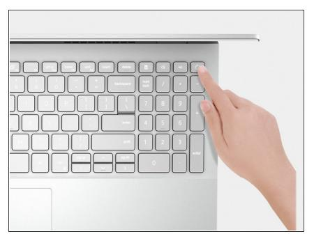
Press and hold the power button for five seconds to ground the computer and drain the flea power.
