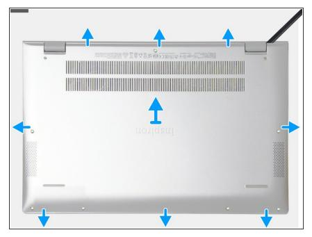
Using a plastic scribe, pry the base cover starting from the recess at the display hinge and work your way around the sides to remove the base cover.
