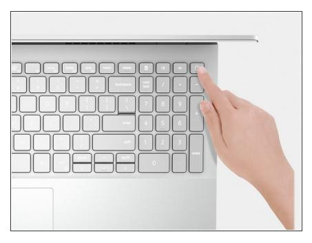
Press and hold the power button for five seconds to ground the computer and drain the flea power. To reassemble your device, follow these instructions in reverse order.
