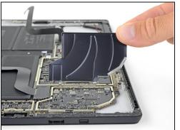
• Repeat the previous step to remove the remaining large EMI shield from the right side of the motherboard.
