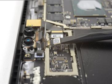
• Use the flat end of a spudger to pry the face-detection camera connector up and out of its socket on the motherboard.
