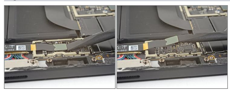
• Use the flat end of a spudger to pry the microSD card reader connector up and out of its socket on the motherboard.
