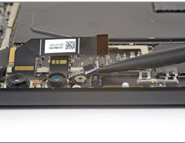
• Use the flat end of a spudger to pry the microphone connector up and out of its socket on the motherboard.
