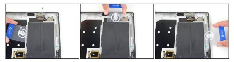
• Repeat the previous two steps for the right side of the battery to release the two right cells from their adhesive.
