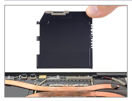
• Remove the heat sink shield.
