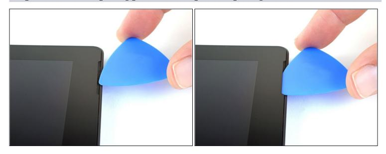
• Insert an opening pick into the speaker opening on the screen and slide the pick under the glass. Do not press the pick into the speaker grille, as the grille is easily torn.
