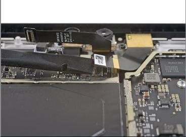
• Use the flat end of a spudger to pry the rear-facing camera connector up and out of its socket on the motherboard.
