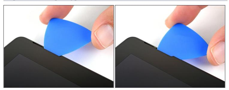
Rotate the pick toward the bottom of the Surface to slide it underneath the lower edge of the speaker cutout.
