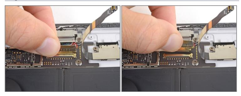
• Slide the SurfaceConnect port connector out of its socket on the motherboard.
