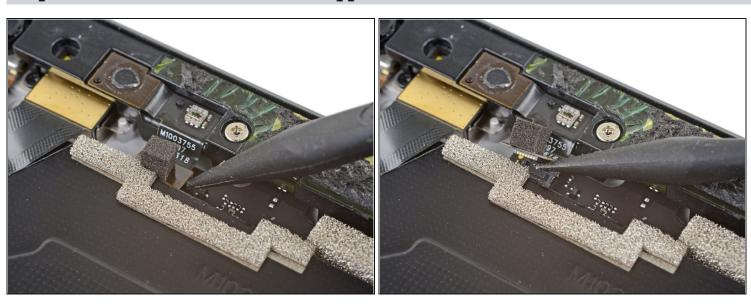
• Use the point of a spudger to pry the microphone connector straight up and out of its socket on the motherboard.
