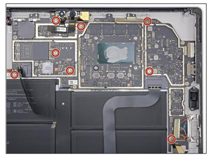
Use a T3 Torx driver to remove the eight 2.2 mm screws securing the motherboard.
