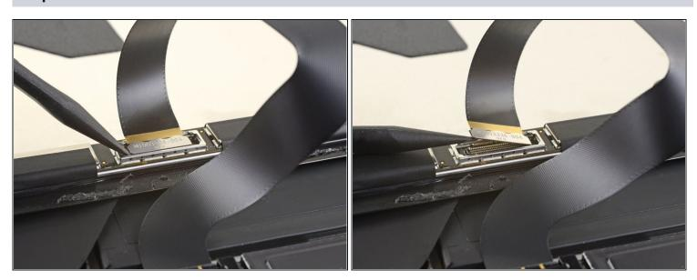
• Use the tip of a spudger to pry the digitizer connector straight up and out of its socket on the screen.
