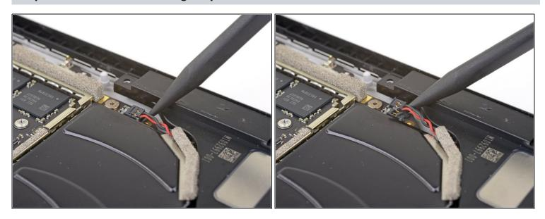
Use the point of a spudger to lift the right speaker connector out of its socket on the motherboard.
