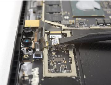
Use the flat end of a spudger to pry the face-detection camera connector up and out of its socket on the motherboard.
