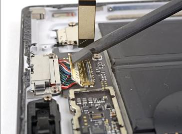
• Use the flat end of a spudger to lift the flap that sits over the SurfaceConnect port connector.
