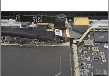
Use the flat end of a spudger to pry the rear-facing camera connector up and out of its socket on the motherboard.
