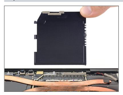
• Remove the heat sink shield.
