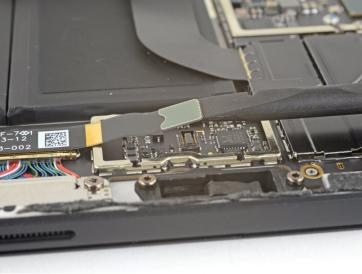
Use the flat end of a spudger to pry the microSD card reader connector up and out of its socket on the motherboard.
