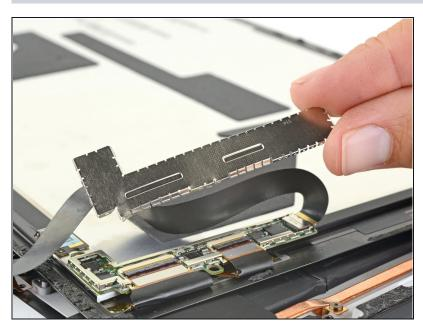
Lift the EMI shield away from the display board and remove it.
