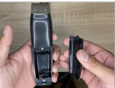
Take out the batteries by pulling off the cover from the back and once done put the cover back on.
