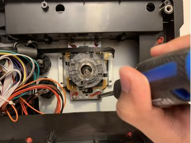
Remove the four 1.1mm screws holding the lever in place with your Phillips #0 screwdriver.
