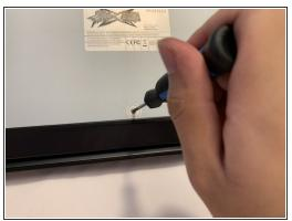
Remove the six 0.9mm screws with a Phillips #00 screwdriver.
