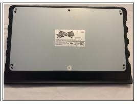
• Remove the four 3mm screws with a Philips #0 screwdriver.
