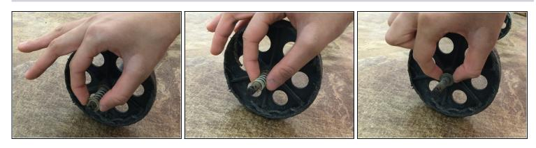
• Slide off the first washer, the spring, and the second washer.
