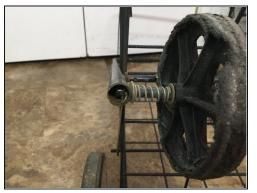
Using a large needle nose plier, take out the stoppers from each side of the axle.
