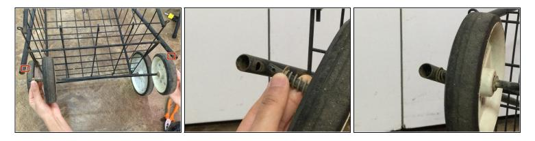
• Carefully place the front wheel axle with the new wheels in the side holes of the cart's legs.
