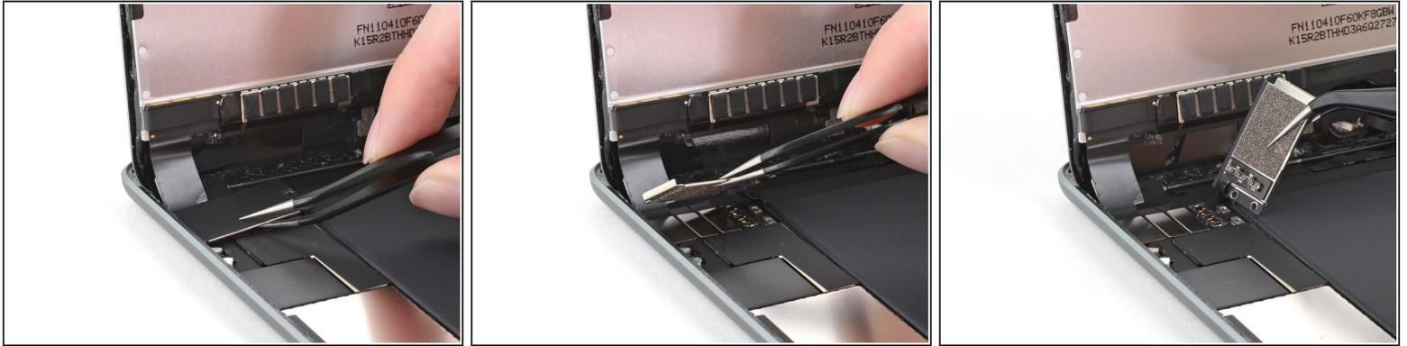
**i** The display cable bracket is secured by a clip under the edge of the frame.
