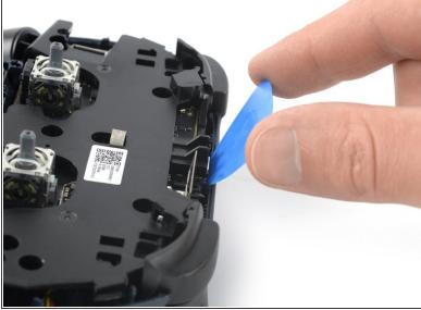
Insert an opening pick at the top edge of the Stadia controller to prevent the charging port from snapping back into place.
