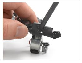
In the following procedure, hold the vibration motor housing as close to the motor as possible.
