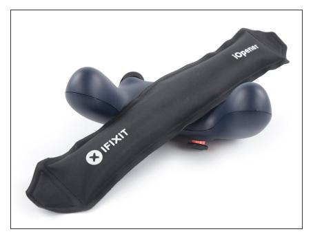
Apply a <u>heated iOpener</u> to the rear side of the Stadia controller where the screw cover is located to loosen the adhesive underneath. Apply the iOpener for at least two minutes.
