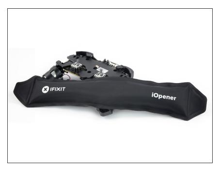
Apply a <u>heated iOpener</u> to the rear side of the right vibration motor to loosen the adhesive underneath.
