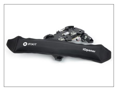
Apply a <u>heated iOpener</u> to the rear side of the left vibration motor to loosen the adhesive underneath.
