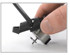
⚠ In the following procedure, hold the vibration motor housing as close to the motor as possible. Otherwise it could bend or break off.
