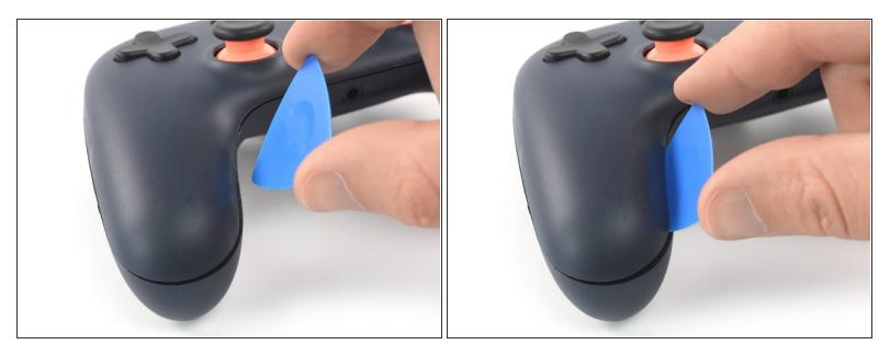
Insert an opening pick in a steep angle into the gap you created to prevent the first clamp from popping back into its closed position.
