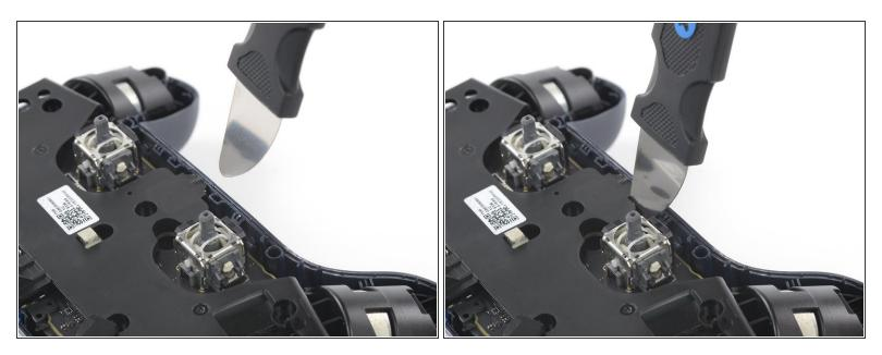
Insert a Jimmy into the gap between the rear cover and the motherboard left of the headphone jack.
