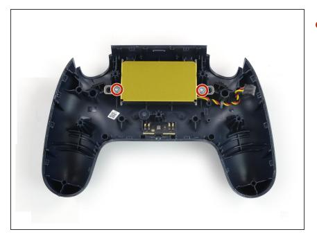
Use a Torx T6 screwdriver to remove the two 6.1 mm-long screws securing the battery.
