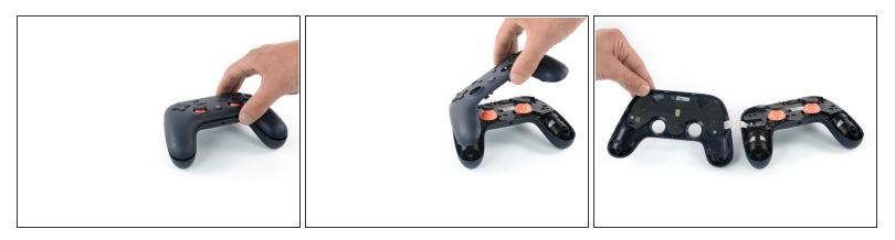
Avoid straining the front cover assembly cable during this step.
