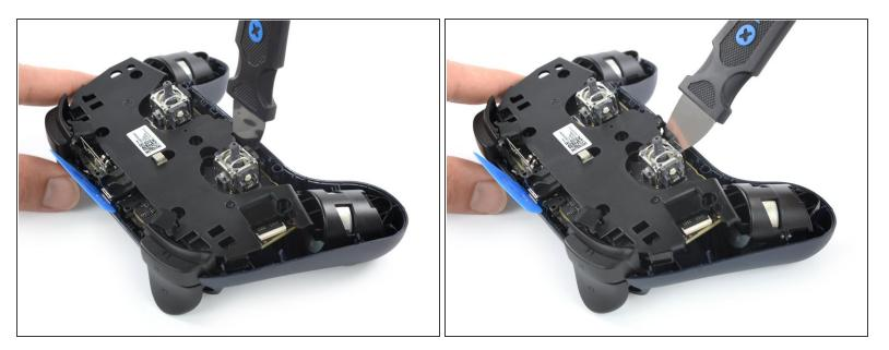
• Pry up the motherboard assembly by tilting the Jimmy downwards.
