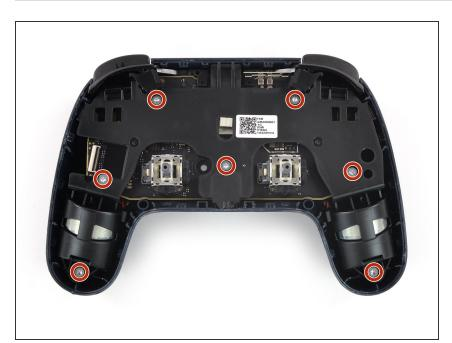
Use a Torx T8 screwdriver to remove the seven 9.6 mm-long screws securing the motherboard assembly.
