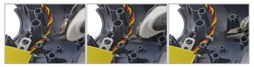
• Use a flush cutter to carefully cut the adhesive holding the battery cable in place.
