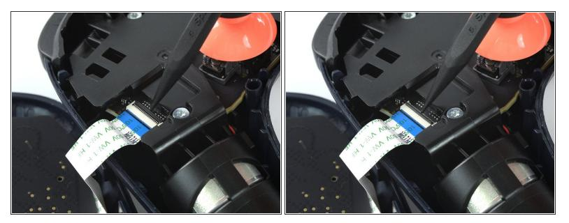
Use the pointed end of a spudger to open the <u>ZIF connector</u> holding the button contact board cable in place.
