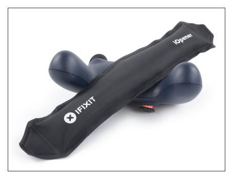
Apply a <u>heated iOpener</u> to the rear side of the Stadia controller where the screw cover is located to loosen the adhesive underneath. Apply the iOpener for at least two minutes.
