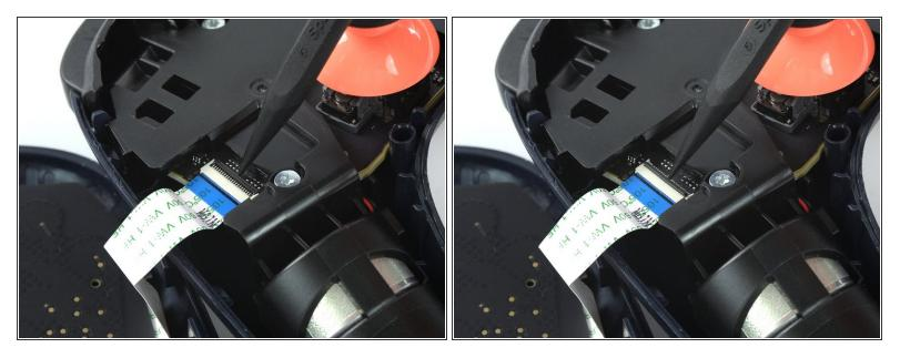
Use the pointed end of a spudger to open the <u>ZIF connector</u> holding the button contact board cable in place.
