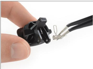
Use a pair of tweezers to remove the spring from the right trigger.
