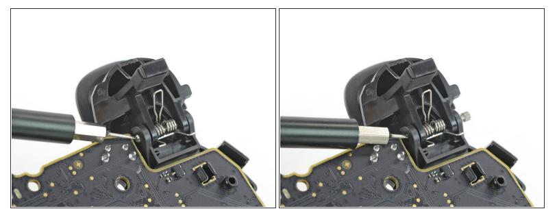
Use a SIM eject bit to push against the inner end of the cylindrical pin holding the right trigger in place.
