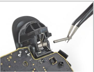
Use a pair of tweezers to pull the cylindrical pin from its guide.
