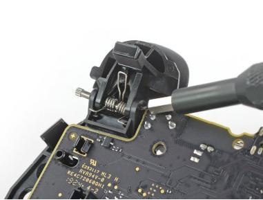
Use a SIM eject bit to push against the inner end of the cylindrical pin holding the left trigger in place.
