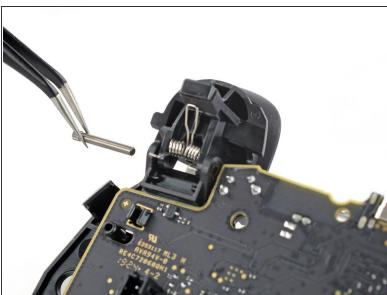
Use a pair of tweezers to pull the cylindrical pin from its guide.
