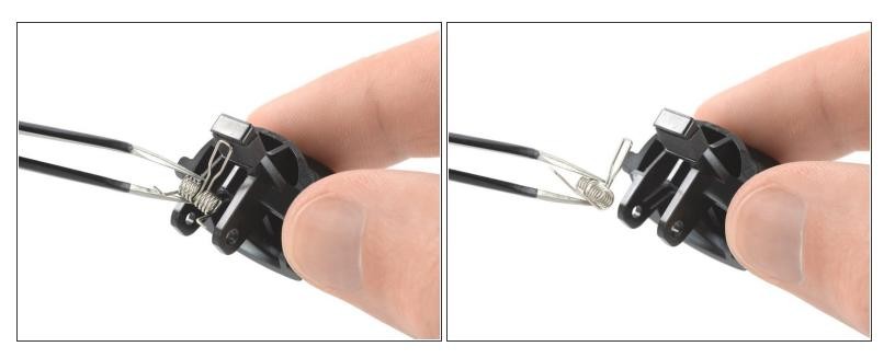
Use a pair of tweezers to remove the spring from the left trigger.
