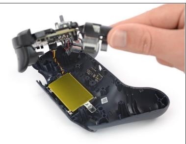
Carefully lift the left edge of the motherboard assembly in order to access the battery connector.
