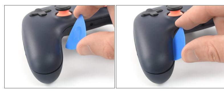
Insert an opening pick in a steep angle into the gap you created to prevent the first clamp from popping back into its closed position.
