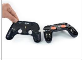
Avoid straining the front cover assembly cable during this step.
