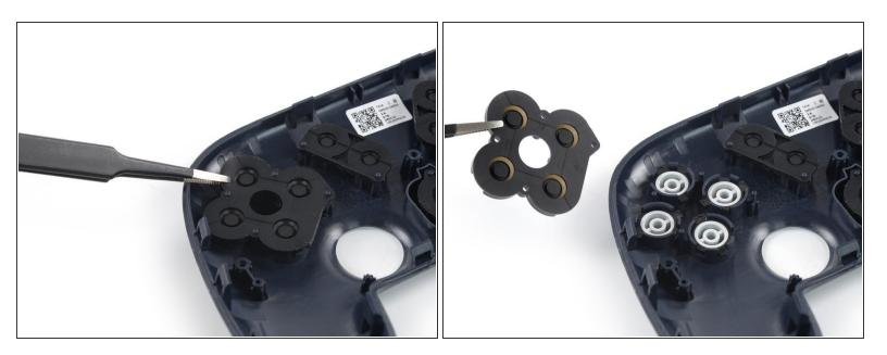
Use a pair of tweezers or your fingers to remove the rubber gasket on the A, B, X and Y buttons.
