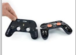
Avoid straining the front cover assembly cable during this step.
