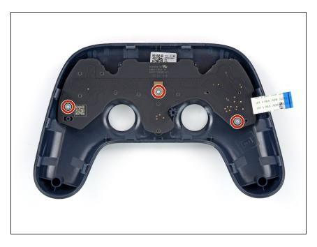
Use a Torx T6 screwdriver to remove the three 6.2 mm-long screws securing the front button contact board.
