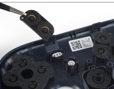
Use a pair of tweezers or your fingers to remove the rubber gasket on the menu and the capture button.
