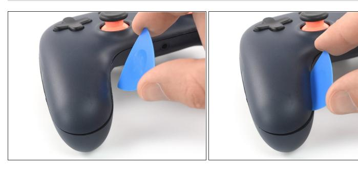
Insert an opening pick in a steep angle into the gap you created to prevent the first clamp from popping back into its closed position.
