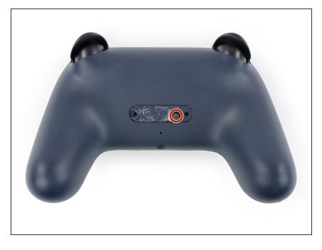
Use a Torx T8 screwdriver to remove the 9.6 mm-long screw securing the rear case.
